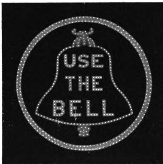
This illuminated Blue Bell sign is now located on the south end of the Company's general office building, at 1230 Arch Street, Philadelphia. The circle is 25 feet in diameter and was so designed to give an appearance at a distance of the standard seal trademark. There are 478 5-watt Tungsten lamps used, 129 of which are blue, forming the outline of the bell. The remaining lamps forming the letters and the circle are white. The sign is seen by northbound travelers on 13th Street and by others in a large radius south of the building.
