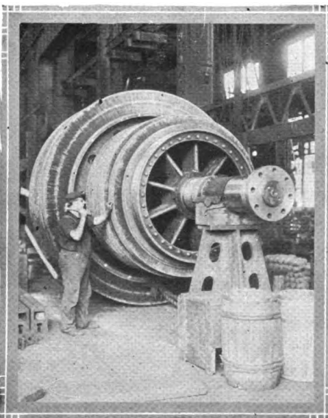
One of the Immense Rotors to be Installed in the Turbines with which the "Wyoming" will be Equipped.
