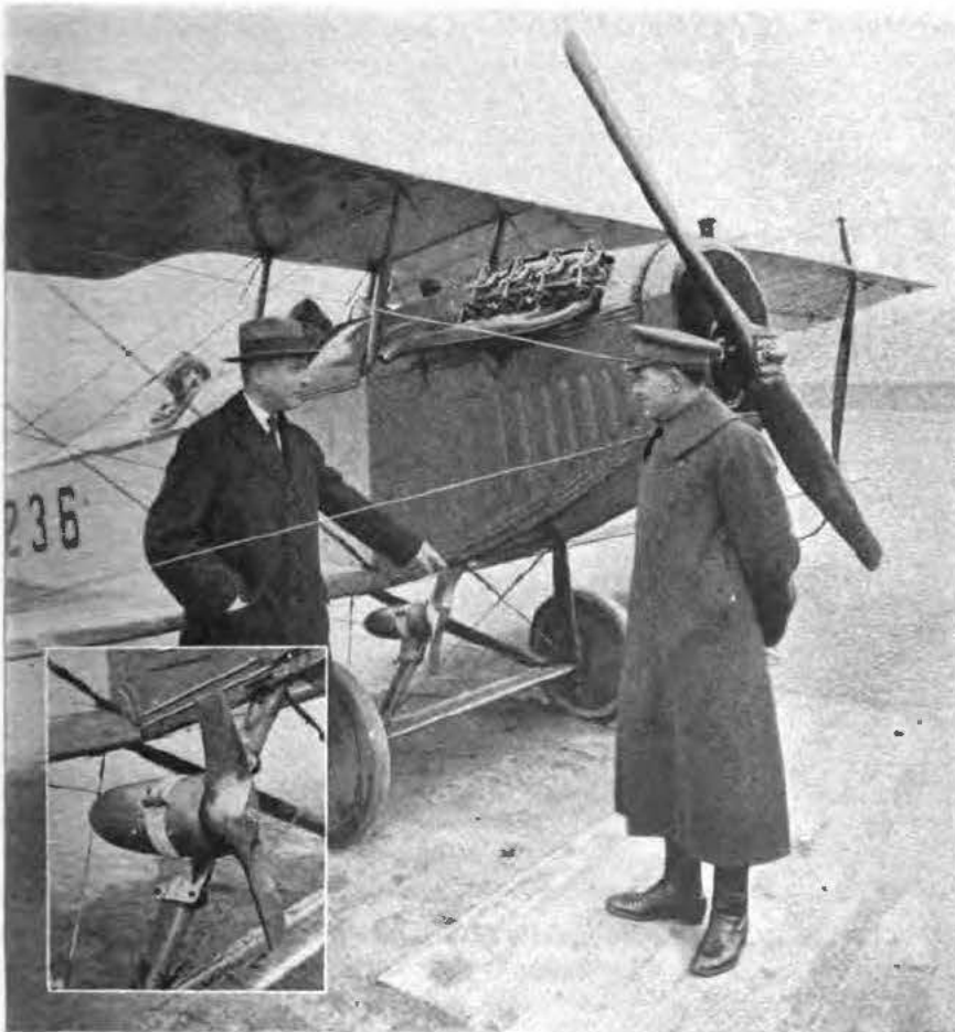
The Wind-Driven Generator Which Supplies the Radio Apparatus. Mr. Craft is Pointing Out Its Position on the Plane, and in the Lower Left-Hand Corner, a "Close Up" of the Generator is Shown
