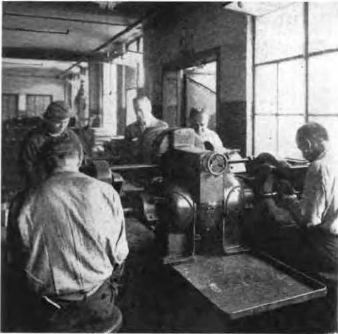
Fig. 8—The last word in polishing and buffing machinery. Dust is exhausted through the pedestal and there are no overhead belts
