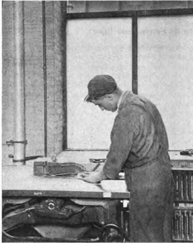
Fig. 3—A circular saw guard that prevents fingers from getting against the saw
