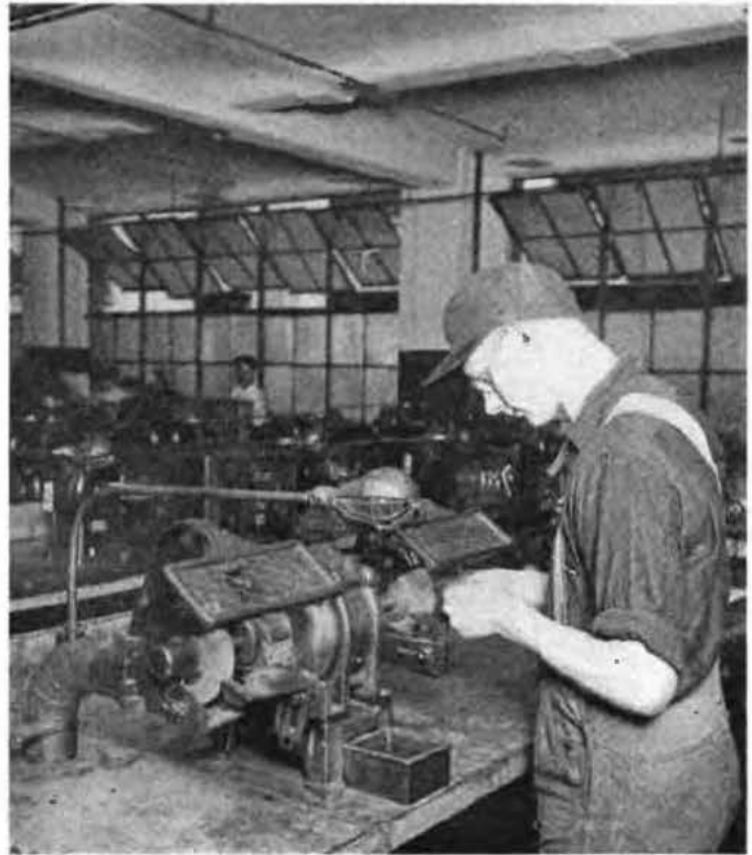
Fig. 9—Bench grinder equipped with exhaust hoods and glass guards
