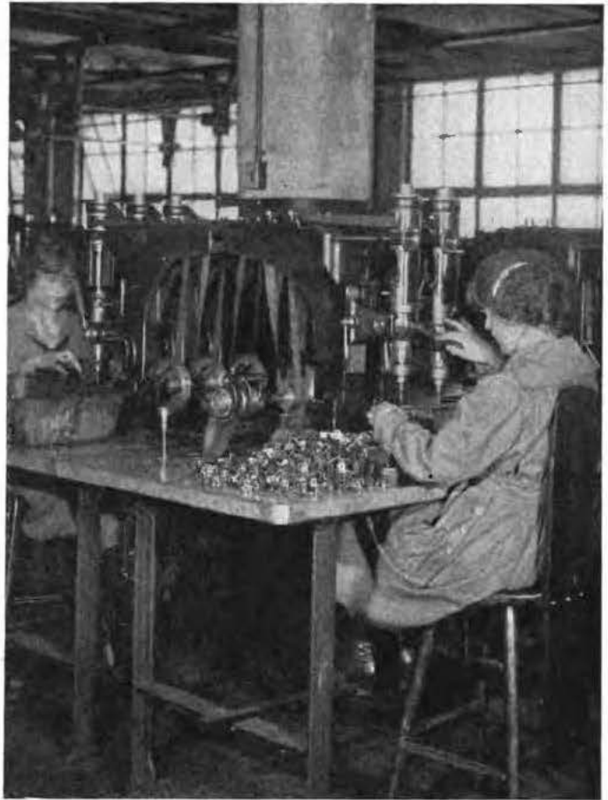
Fig. 2—Showing the method of mounting drill presses back to back, to prevent possibility of injury from the back belts. The horizontal belts driving the drill spindles are protected by the iron guards, which can be seen extending partly around the front pulleys
