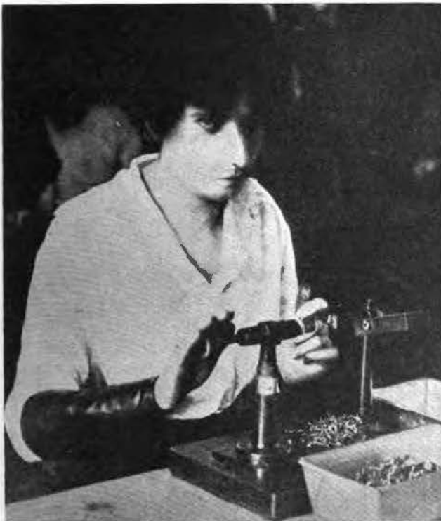
Fig. 3—Assembling the Coil in the Shell
