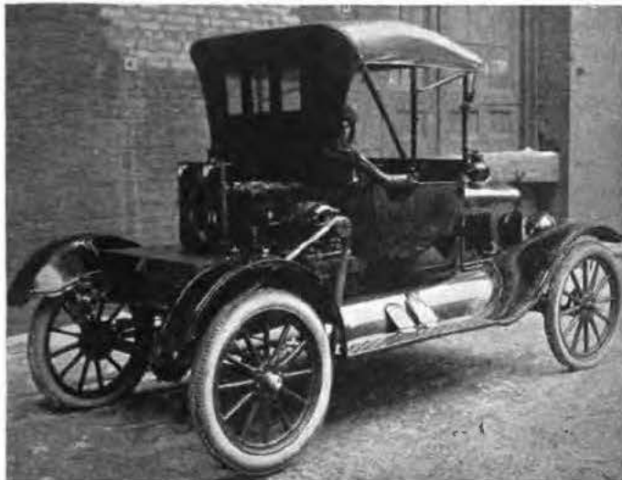
Ford Runabout with a No. 11 Farm Lighting Plant on the Back. To be Used in Demonstrating by Our Chicago House
