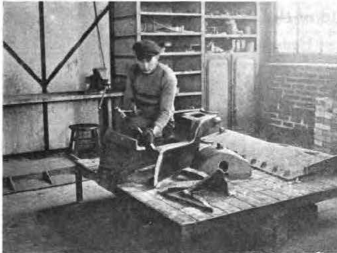
Fig. 1. Chiseling the Break Preparatory to Welding
