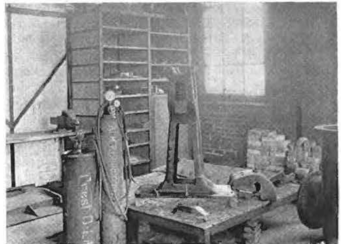
Fig. 3. The Mended Casting, Placed on Two Bricks to Prove Its Strength. The Chalk Marks Show Where the Breaks Were
