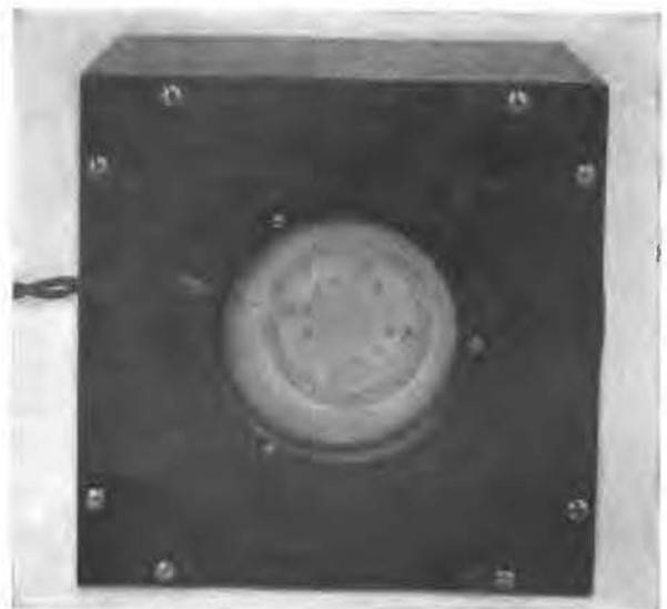
FIGURE 4 Loud Speaking Telephone Transmitter Mounted in Shock-Protecting Case
