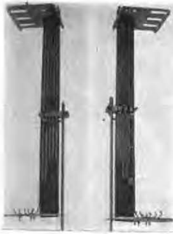
Fig. 6. Commutator for controlling vertical movement of selecting mechanism
