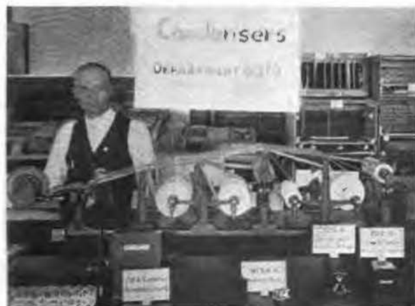
Two strips of tinfoil, insulated by strips of special tissue paper and rolled in a package resembling a miniature bolt of cloth constitutes the essentials of a telephone condenser. This machine winds the strips
