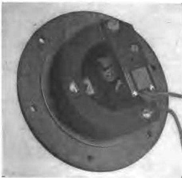
FIGURE 3 Loud Speaking Telephone Receiver Shown With Top of Case Removed
