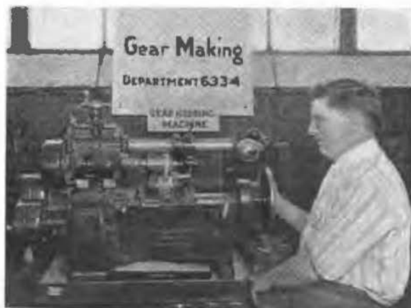
Cutting teeth is a painless and rapid process with this gear hobbing machine. It is here engaged in supplying the dental equipment to hand generator gear blanks
