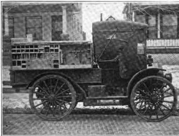
LOOP TRUCK USED BY CLEVELAND PLANT DEPARTMENT. Right side showing general and close view of material box open.
