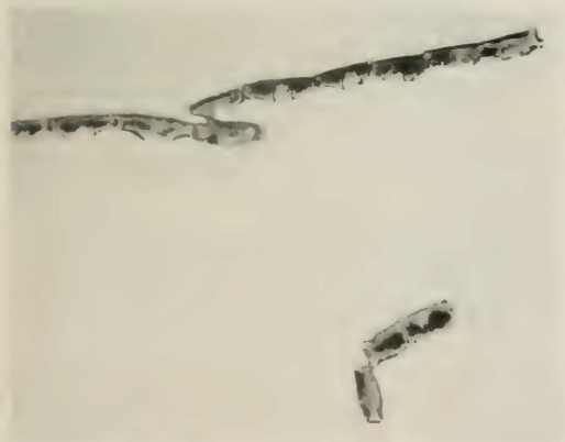
(b) Ash of Manila Hemp, magnification 450 X.
