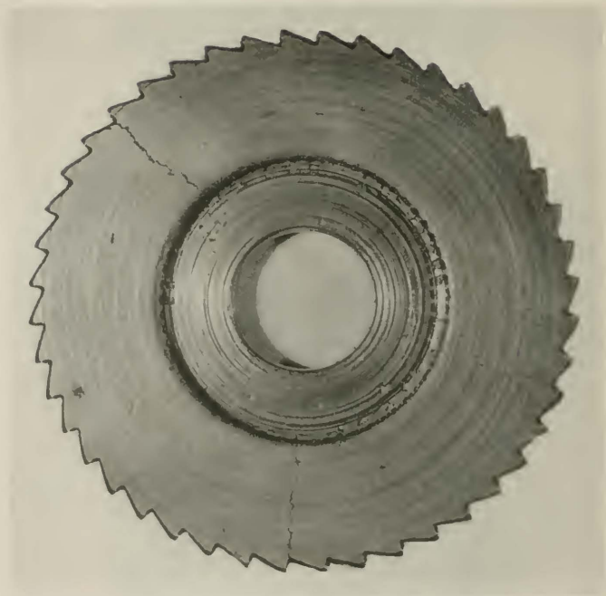
Fig. G. Season cracking of aluminum bronze ratchet wheels. (a) Ratchet wheel at magnification 2\frac{1}{4} X.
