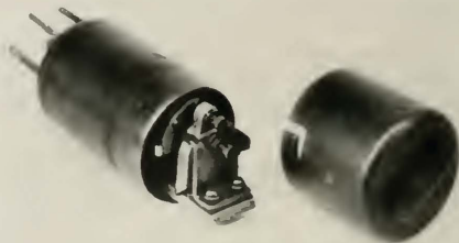
Fig. 7—Early supervisory relay
