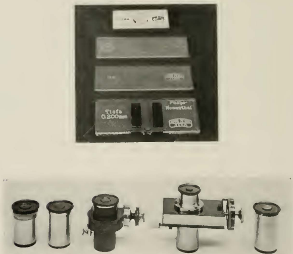
Fig. 26—Various types of eyepiece and stage micrometers used in connection with the microscope to obtain the dimensions of microscopic objects.
