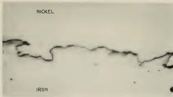
Fig. B. The application of high-power photography to the study of nickel finishes. One of the characteristics of an improved process for plating ductile nickel on iron is the interlocking or "keying" of the nickel and the iron. Magnification, 6000 X.
