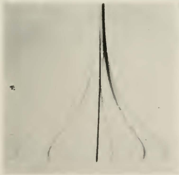
Fig. 11—A group of lines near \lambda 4388 (parhelium spectrum) resolved and spread out in the Crookes dark space. See footnote 15 .
