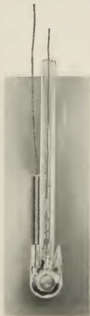
Fig. 2—Photograph of photoelectric cell of type used in picture transmission
