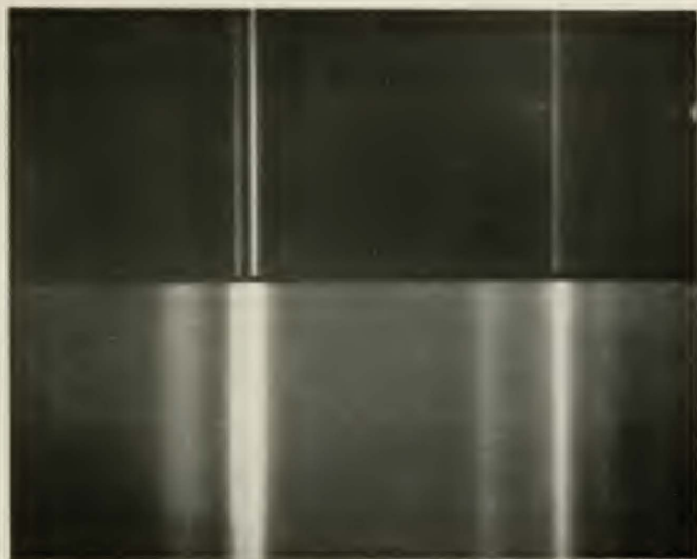
Fig. 7—Above, the K -spectrum of molybdenum ( \alpha -doublet, \beta -line, \gamma -line from left to right); below, the spectrum of this same radiation after scattering at 90^\circ from aluminum (each line doubled). (P. A. Ross)
