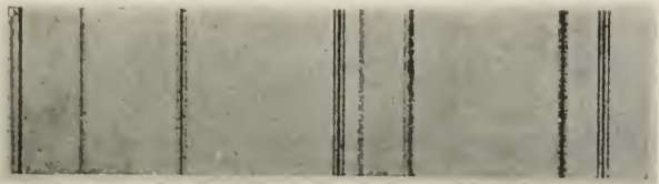
Fig. 9—Effect of magnetic field on spectrum lines. (P. Zeeman, Journal of the Franklin Institute )
