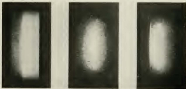
Fig. 8—The Crookes dark space between the cathode (thin line at left) and the negative glow. See footnote 12. (Aston, Proceedings of the Royal Society )
