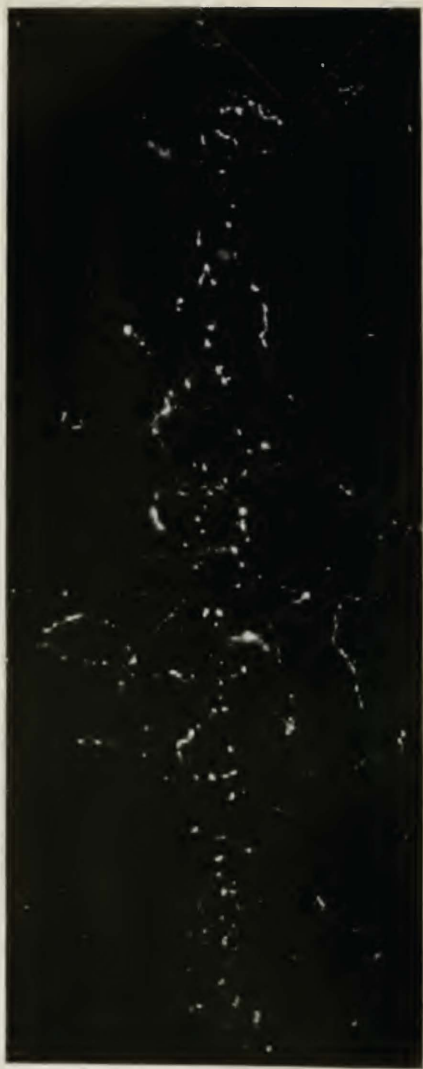
Fig. 10—Trails of recoiling electrons, mingled with long sinuous trails of electrons ejected from atoms by totally-absorbed quanta. (C. T. R. Wilson, Proceedings of the Royal Society )
