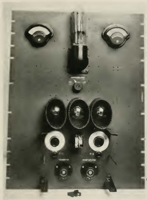
Fig. 6—Front View of Transmitter Panel with Cover Removed from Tuning Condensers
