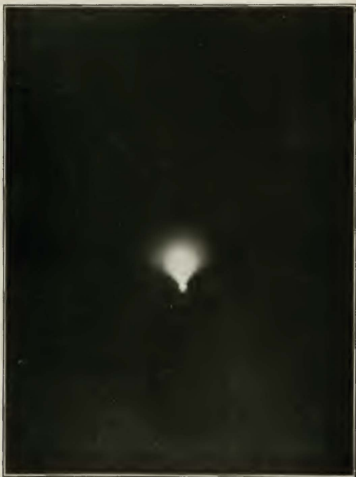
Fig. 13—Magnification of one of the pictures in Fig. 11. (The lowest bright spot is a reflection in the cathode surface)
