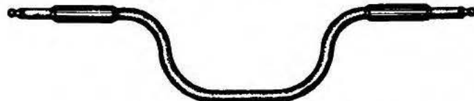
Figure 17. Two Conductor Plug-ended Cords Used to Build up Circuits for Simultaneous Telephony and Telegraphy.
