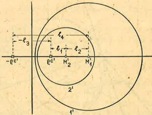
Fig. 5. Dependence of  $a$  upon the double ratio of  $M'_2$  and  $-qc'$  with respect to  $qc'$  and  $M'_1$ .  $1/a = 1 - l_1 l_4 / l_2 l_3$ .
