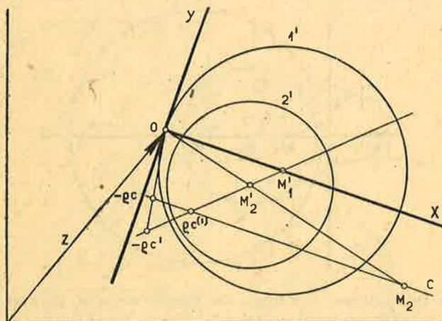
Fig. 4. Circles of 0%,  $a\%$  and 100% absorption in the electrical  $Z_{tot}$ -plane and the proof that  $a$  is independent of the centre of inversion  $O$  on circle  $1'$ .
