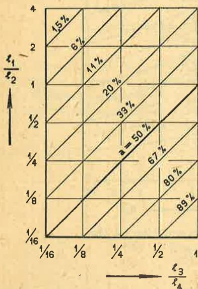
Fig. 6. Graphical representation of the relation between  $a$  and the ratios  $l_1/l_2$  and  $l_3/l_4$ .
